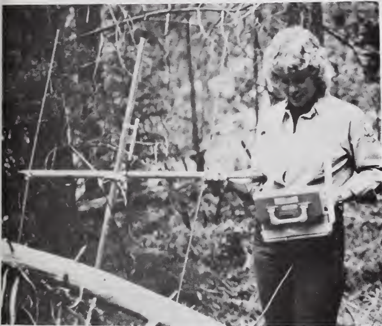
Figure 2.--Portable receiving units can be used with different antenna systems, such as the loop antenna (top) and Yagi antenna (bottom), to locate and observe owls under field conditions.
