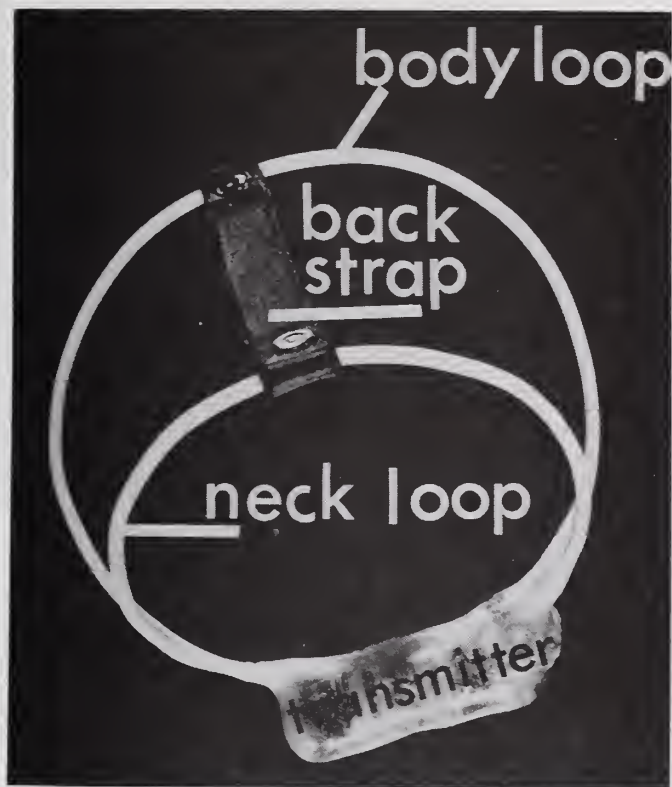
Figure 7.--The first radio transmitter harnesses placed on great horned and barred owls in the early 1960's weighed 70 to 90 grams and transmitted up to 200 days with signals detected for up to 3 miles by the CCNHA radio-tracking towers. Since then, refinements and new technology allow transmitters to be much smaller, lighter, and more reliable.
